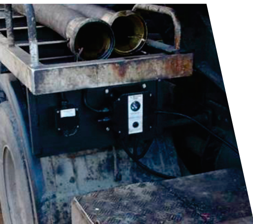
The Earth-Rite II MG static grounding system can be mounted on vacuum trucks and tank trucks.
