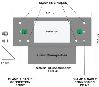
Up to two Newson Gale static grounding clamp and cable assemblies can be connected to the Grounding Station which is then connected to the verified site earth.
