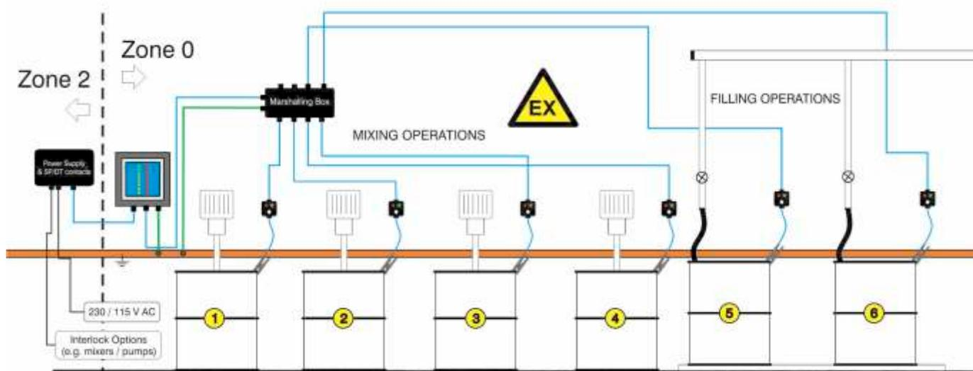
**The Earth-Rite® MULTIPOINT II's monitoring control unit and remote indicator stations can be installed in Zone 0 atmospheres. The power supply unit can be installed in Zone 2 atmospheres.**
