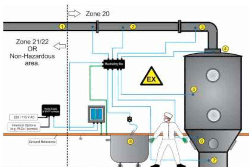
**The Earth-Rite® MULTIPOINT II's monitoring control unit and remote indicator stations can be installed in Zone 20 atmospheres. The power supply unit can be installed in Zone 21 atmospheres. This configuration enables companies employ 24/7 monitoring of interconnected process equipment. This is particularly important when equipment is regularly disassembled and reassembled for cleaning and maintenance activities.**
