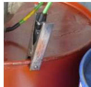
Static grounding clamps must be capable of breaking through coatings, product deposits and rust to ensure a good electrical connection to process equipment.
