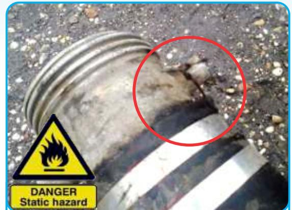
The metal helical wires that reinforce hoses against discharge and suction pressures are commonly used to provide an electrical bond between the end fittings or couplings of hoses. It is important to ensure that wires, like the one illustrated, do not break as this will result in the presence of isolated conductors that have the potential to discharge electrostatic sparks during the material transfer operation.
