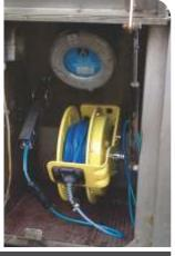
The **VESM02** reel is an alternative to using retractable spiral cable. The NEMA4 housing does a great job of protecting the silver plated slip rings and internal electrical connections. The reel features a ratchet locking mechanism and is supplied with 15 mtr. (50 ft.) of **Cen-Stat™** 2 pole cable.
