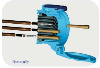
To remove, use the tool provided. Push tool from front onto contact until tool stops. Contact is then released at rear of insulator.
